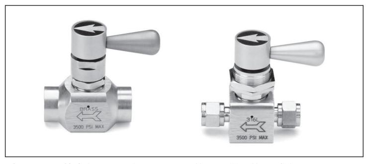
GasFlo Products QSL Series Valves provide quarter turn, positive shut off for critical gas/fluid systems. The lever handle design allows for visual open/closed indication and quick acting cycling. This springless diaphragm valve offers superior leak integrity for Specialty Gas, Chemical, Instrumentation, Semiconductor, Medical and general purpose applications with pressure ranges from vacuum to 3500 psig.
